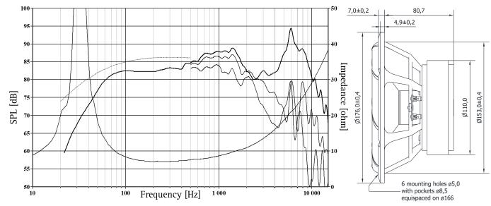
The frequency responses above show measured free field sound pressure in 0, 30, and 60 degrees angle using a 12L closed box. Input 2.83 VRMS, microphone distance 0.5m, normalized to SPL 1m.The dotted line is a calculated response in infinite baffle based on the parameters given for this specific driver. The impedance is measured in free air without baffle using a 2V sine signal.
