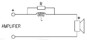
Below you can see the effect of the recommended network on the axial sound pressure frequency response measured in the proposed 19 litre ported enclosure. Black: No network. Red: Inductor L = 1.2 mH, resistor R = 18 Ohms.
