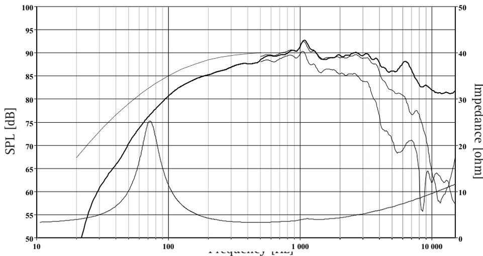
The frequency responses above show measured free field sound pressure in 0, 30, and 60 degrees angle using a 2.5l closed box. Input 2.83 V<sub>RMS</sub>, microphone distance 0.5m, normalized to SPL 1m. The dotted line is a calculated response in infinite baffle based on the parameters given for this specific driver. The impedance is measured in free air without baffle using a 2V sine signal.
