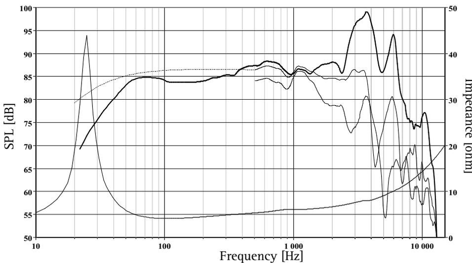
The frequency responses above show measured free field sound pressure in 0, 30, and 60 degrees angle using a 28L closed box. Input 2.83 V<sub>RMS</sub>, microphone distance 0.5m, normalized to SPL 1m. The dotted line is a calculated response in infinite baffle based on the parameters given for this specific driver. The impedance is measured in free air without baffle using a 2V sine signal.
