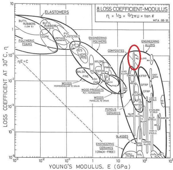
A classical benchmark for loudspeaker cone materials is the stiffness-to-weight ratio, which gives you the speed of sound in the material. Higher is better. See graph on the right side, magnesium is marked as a red dot:
