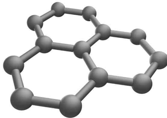
Graphene must be dispersed evenly and not clog together, because then it loses its properties and instead retains the properties of Graphite (nick named fake Graphene).
